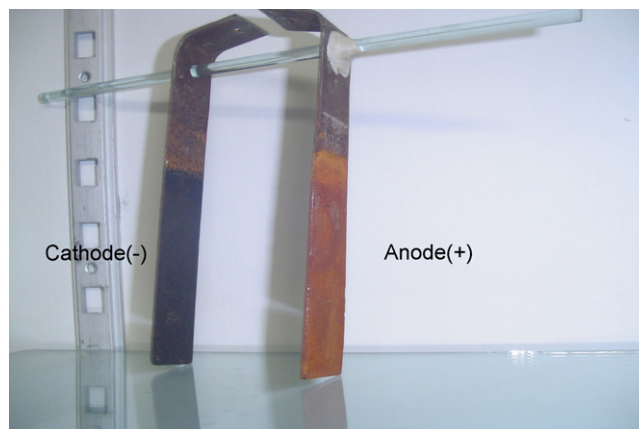
Fig. 9. Electrodes after the experimental run. Top portions of electrodes show initial conditions (prior to EC).
